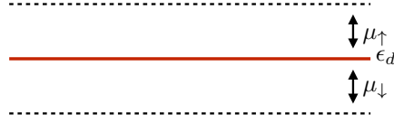
Fig. 14: A net magnetization gives rise to spin-dependent chemical potentials in the quantum dot.
