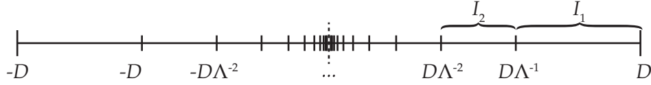
Figure III.8: Sketch of the logarithmic discretization. The full band [-D, D] is divided into energy intervals, the size of which scales with \Lambda^{-n} .
