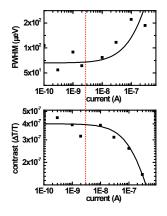
Figure S5: The peak contrast and linewidth of dot 1 as a function of the laser intensity.
