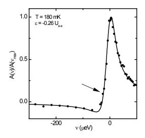
Figure S1: For  $\nu < -T$ , the red side (arrow) of the absorption resonance has a strong dependence on the temperature T. Dots: experimental data. Line: NRG prediction, obtained via Eq. (S2) as described in Sec. S2, using the temperature T as fit parameter.
