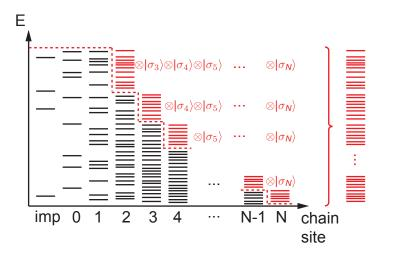
Figure 4.3.: Eigenenergies obtained from the NRG algorithm. The discarded states (red) constitute a complete and orthonormal basis. The environmental states  $|\sigma_n\rangle$  indicate that the discarded states are no longer refined but that they are considered to be appropriately degenerate instead, which is reflected in their weighting factors at the calculation of the spectral function (c. f. Eq. (4.31)). Figure adapted from [43].
