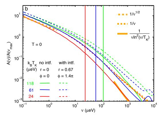
Figure S3: NRG results for the T = 0 line shapes of Fig. 3b shown with interference effect as in the main text (dashed lines), and without (solid lines).
