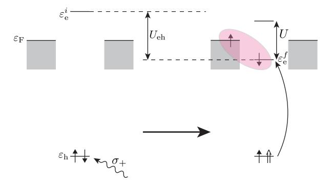
Figure 3.3.: Schematic picture of the excitonic Anderson model with Kondo correlations in the final state. After absorption, the local level is in a position such that it is occupied by a single electron, which can build a Kondo state with the surrounding reservoir electrons.
