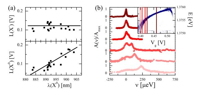
FIG. S4. (a) Gate voltage extents (lengths) of the  $X^-$  and the  $X^0$  plateaus of all studied QDs extracted from photoluminescence measurements. The black lines are a guide to the eye. (b) An example of the double peak structure in a different dot that has smaller tunnel coupling. Inset: 2D differential transmission scan of the  $X^0$  plateau together with the indicated positions of the measured absorption line shapes.
