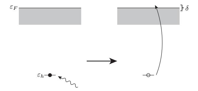
Figure 3.2.: Schematic picture of the absorption process which leads to the Fermi edge singularity. At absorption of a photon, an electron from an inner shell is lifted above the Fermi level. Due to the potential of the resulting core hole, the electrons at the Fermi level acquire a phase shift and the resulting (divergent) absorption spectrum can be explained by Anderson orthogonality.
