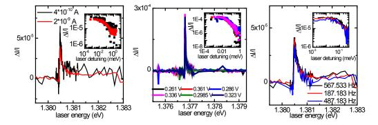
Figure S4: Dependence of the line shape on measurement parameters: Left: intensity dependence of the line shape; the intensity I is depicted in terms of the current it produces in the photodiode; an incident intensity of 10 nW produces a current of 4 nA. Middle: modulation voltage dependence. The gate voltage is modulated with a square-wave between 0.311 V and the values depicted in the figure. Right: lock-in modulation frequency dependence of the absorption line shape.
