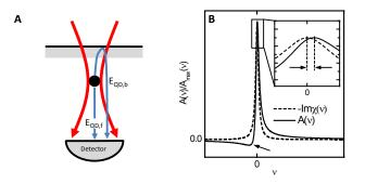
Figure S2: **a**, Schematic of the origin of the interference effect. **b** Effect of the interference on a Lorentzian line shape. NRG results for the T = 0 line shapes of Fig. 3b shown with interference effect as in the main text (dashed lines), and without (solid lines).
