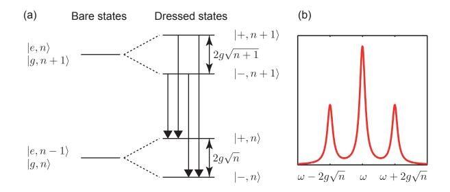
Figure 3.6.: Schematic of the transitions that yield the Mollow triplet and qualitative behavior of the RF spectrum. (a) shows the possible transitions between the dressed states of two neighboring manifolds. Two of the four possible transitions have the same frequency, which for  $T \gg \Omega$  causes the emission to be twice as strong for this frequency as for the other transitions (b). Figure adapted from [66].
