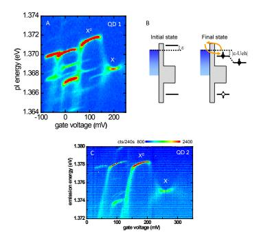
Figure S7: (a) Photoluminescence as a function of  $V_g$  for dot 1: this is the same plot as in Fig. 1b of the main text. (b) Schematic of the  $X^0$  transition. The  $X^0$  plateau has a curvature with a different sign as compared to  $X^-$ , since the renormalization of the electron level energy  $\varepsilon_{e\sigma}$  by hybridization with the FR is relevant only in the final state. (c) Photoluminescence as a function of  $V_g$  for dot 2.
