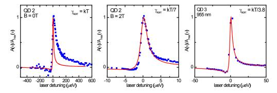
Figure S6: Perturbative fits to absorption line shapes measured for (a) dot 2 at B = 0 Tesla, (b) dot 2 at B = 2 Tesla, (c) dot 3 at B = 0 Tesla.
