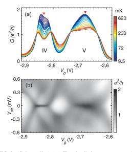
FIG. 3. (Color online) (a) The detailed measurement of the conductance temperature dependence shown in Fig. 1(c), valleys IV and V. The red triangles mark two values of  $V_g = -2.835$  and -2.680 V for which the conductance as a function of  $V_{sd}$  is plotted in Figs. 4(a) and 4(b), respectively. (b) The gray-scale conductance plot in the  $V_g$ - $V_{sd}$  plane was measured in the same range of  $V_g$  as in (a), at temperature T = 10 mK.
