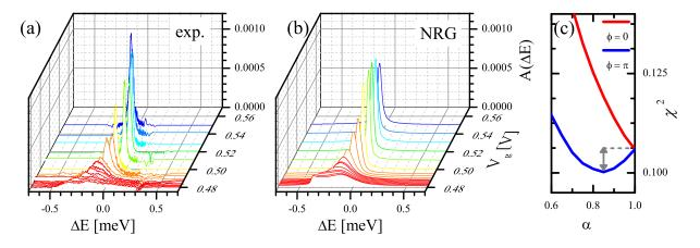
FIG. S6. Comparison of measured line shapes (a) and NRG simulations (b) in the gate voltage range of  $V_g = 0.48$  V to 0.55 V (not normalized, cf. Fig. 1(c)) (c) Calculated cumulative  $\chi^2$  of all measured line shapes from  $V_g = 0.481$  V to 0.55 V for destructive interference ( $\phi = \eta$ , red) and constructive interference ( $\phi = \pi$ , blue) as a function of branching ratio  $\alpha$ .
