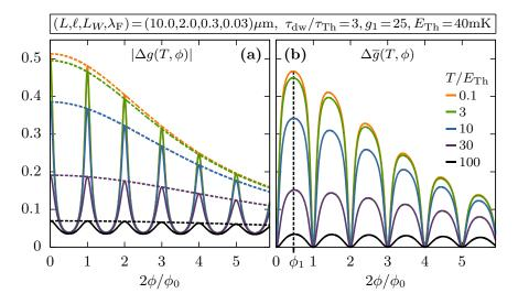
Fig. 1.7. (a) The WL correction  $|\Delta g(T,\phi)|$  (solid lines), its envelope  $|\Delta g_{\rm en}(T,\phi)|$  (dashed lines) and (b) their difference  $\Delta \overline{g} = |\Delta g_{\rm en}| - |\Delta g|$ , plotted as function of magnetic flux  $2\phi/\phi_0$ , for five different temperatures between  $0.1E_{\rm Th}$  and  $100E_{\rm Th}$  (increasing from top to bottom).
