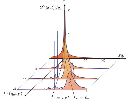
**Figure 2.** Numerical evaluation of  $|G^{>}(x,t)|$  at zero temperature T=0 resulting from bosonization, as a function of x and t (solid blue lines). The weight of the sharp peak at  $x=v_{\rm F}t$  decreases for increasing propagation times t. The dashed blue line shows an approximation of the GF (see equation (42)) which yields good qualitative agreement with the full solution. The plot is done for  $U_q=U_0{\rm e}^{-(q/q_c)^2}$  with  $\frac{U_0}{v_{\rm F}}=2\pi\alpha=5$ .
