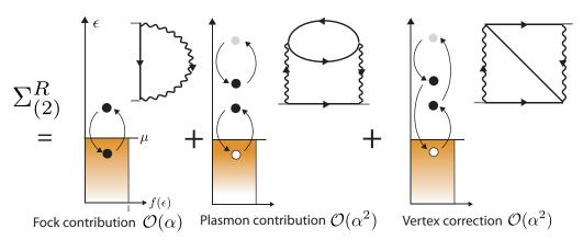
**Figure 7.** The relevant processes which contribute to the self-energy up to second order in the coupling. The wiggly lines indicate the interaction. Note that the plasmonic diagram and the vertex correction differ only by an additional exchange process. That produces a minus sign, such that the diagrams tend to cancel each other at low momenta.
