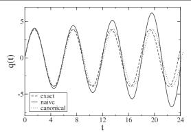
**Figure 1.** We compare the different approaches to solve the equations of motion for the anharmonic oscillator from equation (1). The difference between the numerically exact solution and canonical perturbation theory according to equation (11) can hardly be noticed. Naive perturbation theory already yields large errors after a few oscillations, with an error that grows linearly in time t. Our parameters are v = 4 and coupling strength g = 0.01.
