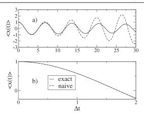
**Figure 3.** Comparison of the exact solution equation (38) against the naive perturbation theory of equation (34). The secular term occurring in the second order perturbation expansion yields an error growing  $\propto t$ , see (a). In the short time limit  $t \ll 1$ , naive perturbation theory becomes exact, see (b). Parameters:  $a = \frac{1}{\sqrt{2}}$ ,  $\Delta = 1$ ; ohmic bath:  $J(\omega) = 2\alpha\omega\Theta(\omega_{\rm c} - \omega)$  with  $\alpha = 0.001$ ,  $\omega_{\rm c} = 10$ .
