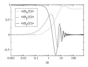
**Figure 6.** Real-time evolution of the spin expectation values  $\langle \sigma_{x,y,z} \rangle(t)$  starting from a polarized spin in the z-direction with a relaxed ohmic bath. We used a damping strength  $\alpha=0.1$  and the parameters N=2000,  $\Delta=1$ , T=0 and  $\omega_{\rm c}=10$ .
