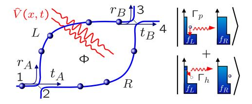
Fig. 1 – (Color online) Left: schematic of the Mach-Zehnder setup. Right: particle- and hole-scattering processes contributing to the dephasing rate, see discussion after eq. (14).
