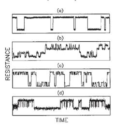
Figure 20. Resistance versus time in copper nanobridges for  $T < 150 \,\mathrm{K}$  showing several types of behaviour. The fluctuations range from 0.005% to 0.2% of the total resistance. The time-scales depend on the temperature at which the fluctuation is observed. (a) A single TLF. (b) Two independent TLFs. (c) Amplitude modulation. (d) Frequency modulation of one TLS by another. [Taken from [94], with kind permission of the American Institute of Physics].
