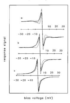
Figure 26. RF response signals at 60 GHz (thick solid line) and 0.6 GHz (dashed line) and d<sup>2</sup>V/dI<sup>2</sup>(V) dependence (thin solid line) for (a) a 26 Ω Fe<sub>80</sub>B<sub>20</sub> point contact, (b) a 8 Ω Fe<sub>78</sub>Mo<sub>2</sub>B<sub>20</sub> point contact, and (c) a 15 Ω Fe<sub>32</sub>Ni<sub>36</sub>Cr<sub>14</sub>P<sub>12</sub>B<sub>6</sub> point contact. [Taken from [103], with kind permission of the American Institute of Physics].
