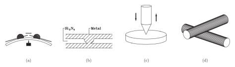
Figure 2. The four main techniques for establishing point contacts. (a) Mechanically controllable break junction, (b) nanoconstriction, (c) spear—anvil geometry, (d) two touching wires.
