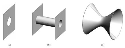
Figure 3. Three point-contact models. (a) An orifice with diameter *d* in an insulating screen between two metallic half-spaces. (b) Two bulk regions are connected with a long, narrow conducting neck. (c) Rotational hyperboloid.
