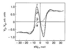
Figure 27. Evolution of the PC spectra of a contact of the annealed alloy  $Ni_{59}Nb_{41}$  with Ag in measurements at different frequencies: a sonic frequency (1) and microwave frequencies  $\omega = 0.48\,\text{GHz}$  (2), 2.036 GHz (3), and 4.72 GHz (4). The anomaly is strongly suppressed with the microwave irradiation, whereas the ZBA in unannealed samples is unaffected by the same irradiation. [Taken from [106] with kind permission of the American Institute of Physics].
