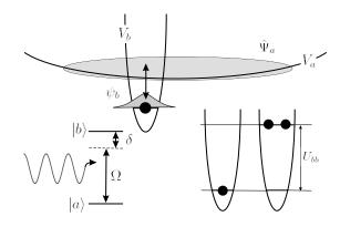
FIG. 1. Schematic setup of an atomic quantum dot coupled to a superfluid atomic reservoir. The Bose liquid of atoms in state a is confined in a shallow trap  $V_a(\mathbf{x})$ . The atom in state b is localized in tightly confining potential  $V_b(\mathbf{x})$ . Atoms in states a and b are coupled via a Raman transition with effective Rabi frequency  $\Omega$ . A large on-site interaction  $U_{bb}>0$  allows only a single atom in the dot.
