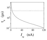
Fig. 7. The dephasing time (42) as a function of the bias current  $I_{sq}$  through the SQUID (solid line). The dashed line shows  $\tau_{\phi}$  for  $I_{sq} = 5$  nA, a typical minimum value for the effective bias current for a SQUID with a few percent asymmetry between its junctions. At this point  $\tau_{\phi} = 131 \ \mu s$ , and  $\alpha = 1 \times 10^{-7}$ . Parameters are further as described in the caption of Figure 5.
