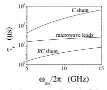
Fig. 6. Typical relaxation times due to the *C*-shunted SQUID, the *RC*-shunted SQUID, and coupling the microwave leads as a function of the resonance frequency at which the qubit is operated. The example of the microwave leads contribution is for a mutual inductance  $M_{mw}$  to the coaxial line of  $M_{mw} = 0.1$  pH. Parameters are further as described in the caption of Figure 5.
