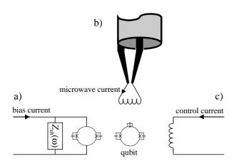
Fig. 1. Experimental setup for measurements on a Josephson persistent-current qubit. The qubit (center) is a superconducting loop that contains three Josephson junctions. It is inductively coupled to a DC-SQUID (a), and superconducting control lines for applying magnetic fields at microwave frequencies (b) and static magnetic fields (c). The DC-SQUID is realized with an on-chip shunt circuit with impedance  $Z_{sh}$ . The circuits a)–c) are connected to filtering and electronics (not drawn).
