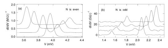
Fig. 8. dI/dV vs. V at 50 mK and H = 0.03, 1, 2, 3 T from bottom to top, for two different samples [5]. The first transition above the Coulomb-blockade threshold exhibits Zeeman splitting in (a) but not in (b), hence the electron number N of the V = 0 ground state is even for grain (a) and odd for grain (b).
