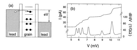
Fig. 3. (a) Cartoon of an dI/dV-measurement: The number of available transport channels through discrete states (here three) is determined by the bias voltage V. (b) The current and differential conductance as functions of bias voltage V for one of RBT's ultrasmall grains; beyond the Coulomb-blockade threshold at around 5.5 mV, the current displays fine steps and the conductance fine peaks, on a voltage scale of a few mV, reflecting the grain's discrete eigenspectrum.
